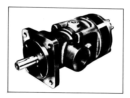
**500 SERIES AXIAL PISTON CONSTANT VOLUME PUMP**  The hydraulic pump mechanism is enclosed in a meehanite housing consisting of three parts: the port block, the body, and the end cap. The port block incorporates the shaft assembly and consists of two preloaded angular contact bearings spaced far enough apart to insure rigidity to the outboard portion of the shaft. A lip type seal held in place by a removable seal retainer effectively prevents leakage around the shaft.
