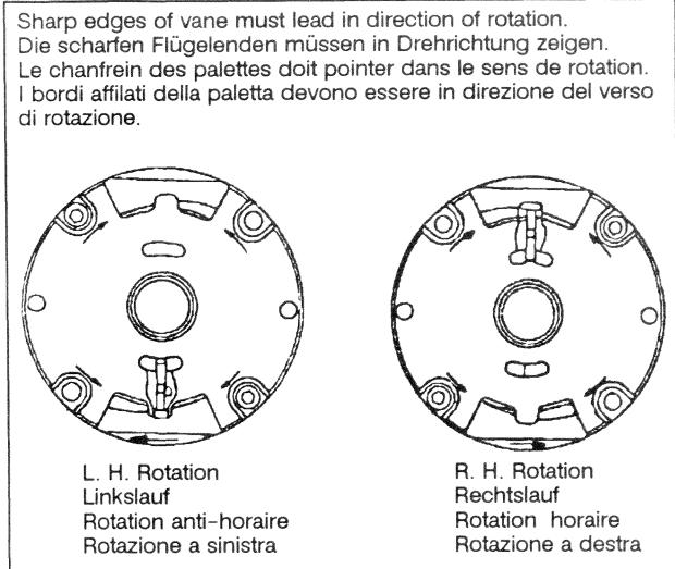
Sharp edges of vane must lead in direction of rotation.
