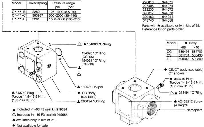
□ NOTE: These parts used at final test to obtain correct pressure range.
