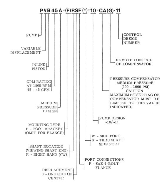
For satisfactory service life of these components in industrial applications, use full flow filtration to provide fluid which meets ISO cleanliness code 16/13 or cleaner. Selections from Vickers OFP, OFR, and OFRS series are recommended.
