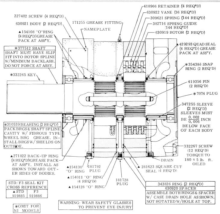
CAUTION: WHEN ASSEMBLING CARTRIDGE, INSERT VANES IN ROTOR SLOTS AT THE MINOR DIA-METER OF CAM RING. ROTATE CARTRIDGE ONE COMPLETE REVOLUTION PRIOR TO ASSEMBLY WITH BODIES. THIS PREVENTS MISALIGNMENT OF SPRINGS AND GUIDES. MAKE SURE THE MARK-ED ROTOR TOOTH OF EACH CARTRIDGE IS IN LINE BEFORE INSTALLATION OF SHAFT.
