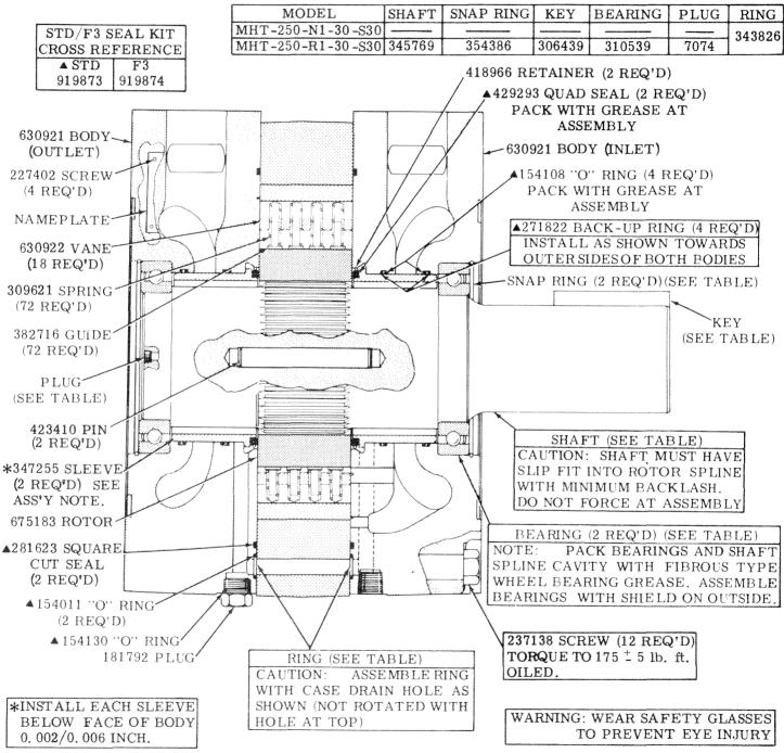
CAUTION: WHEN ASSEMBLING CARTRIDGE. INSERT VANES IN ROTOR SLOTS AT THE MINOR DIAMETER OF CAM RING, ROTATE CARTRIDGE ONE COMPLETE REV-OLUTION PRIOR TO ASSEMBLY WITH BODIES. THIS PREVENTS MISALIGNMENT OF SPRINGS AND GUIDES.
