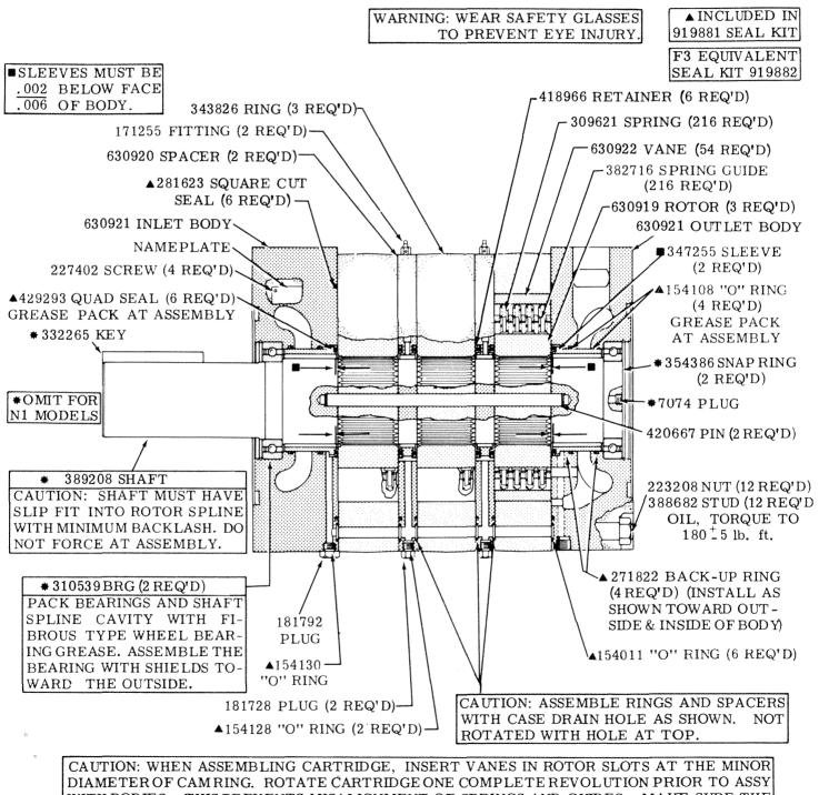
WITH BODIES. THIS PREVENTS MISALIGNMENT OF SPRINGS AND GUIDES. MAKE SURE THE MARKED ROTOR TOOTH OF EACH CARTRIDGE IS IN LINE BEFORE INSTALLATION OF SHAFT.
