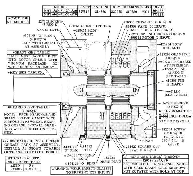
CAUTION: WHEN ASSEMBLING CARTRIDGE, INSERT VANES IN ROTOR SLOTS AT THE MINOR DIA-METER OF CAM RING. ROTATE CARTRIDGE ONE COMPLETE REVOLUTION PRIOR TO ASSEMBLY WITH BODIES. THIS PREVENTS MISALIGNMENT OF SPRINGS AND GUIDES. MAKE SURE THE MARK-ED ROTOR TOOTH OF EACH CARTRIDGE IS IN LINE BEFORE INSTALLATION OF SHAFT.
