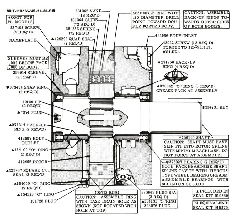
CAUTION: WHEN ASSEMBLING CARTRIDGE, INSERT VANES IN ROTOR SLOTS AT THE MINOR DIAMETER OF CAM RING. ROTATE CARTRIDGE ONE COMPLETE REVOLUTION BY HAND PRIOR TO ASSY WITH BODIES TO PREVENT MISALIGNMENT OF SPRINGS AND GUIDES.
