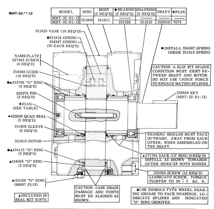
CAUTION: WHEN ASSEMBLING CARTRIDGE, INSERT VANES IN ROTOR SLOTS AT THE MINOR DIAMETER OF CAM RING. ROTATE CARTRIDGE ONE COMPLETE REVOLUTION PRIOR TO ASSY WITH BODIES. THIS PREVENTS MISALIGNMENT OF SPRINGS AND GUIDES.
